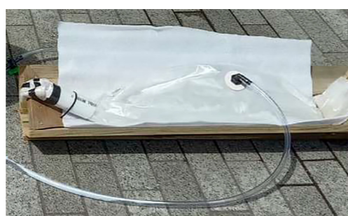
A Plug Flow Digester
