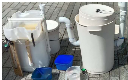
A small Chinese Fixed Dome Digester (left) and an Indian Floating Drum Digester (right)
