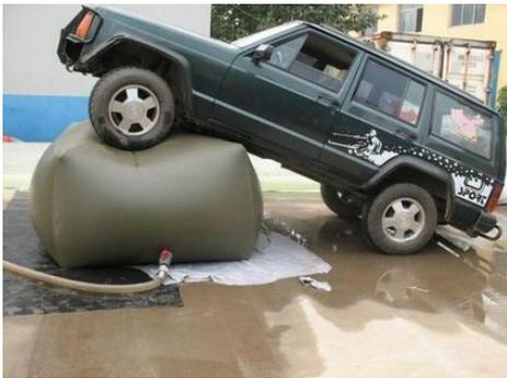
of biogas digester is about 2 kpa, and the Red Mud soft biogas digester can withstand 10 kpa. So there's nothing to worry about.
