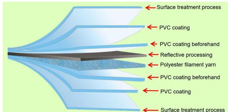
resistance, low temperature flexibility; Flame retardant, heat stability, acid and alkali corrosion resistance, especially excellent waterproof, corrosion resistance and tensile performance. So it's very safe to put in outdoor, and it's durable than other materials commonly.
